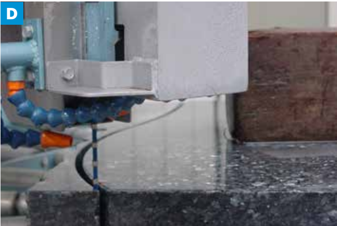
EN Accurate pneumatically controlled cable tensionning.
